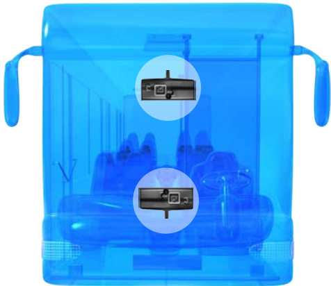
Optional camera mounting positions - top or bottom with 180° panoramic rotation
