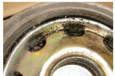
Figure 2: Desiccant cartridge with coalescence filter after 60,000 km
