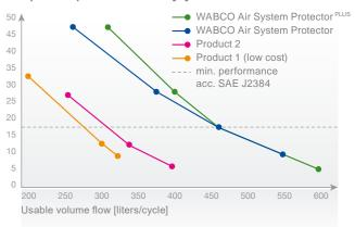
Test conditions: Drying performance test rig of coalescing cartridges acc. SAE J2384; mechanical air dryer with regeneration tank of 6 liters, cut-in: 11 bar, cut-out: 12 bar
