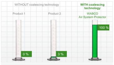
Test conditions: 704 cm<sup>3</sup>-two-cylinder-compressor at high temperature setting 12.5 bar and 50% duty cycle: calculation based on aerosol measurement downstream the air-drver
