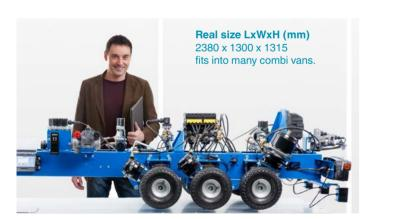
trailer technology. Trailer Training Model features the most up-to-date braking and suspension systems on a scaled down trailer test bed, engineered specifically for use as a
